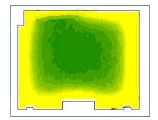
Floor plate designed for maximum light penetration
